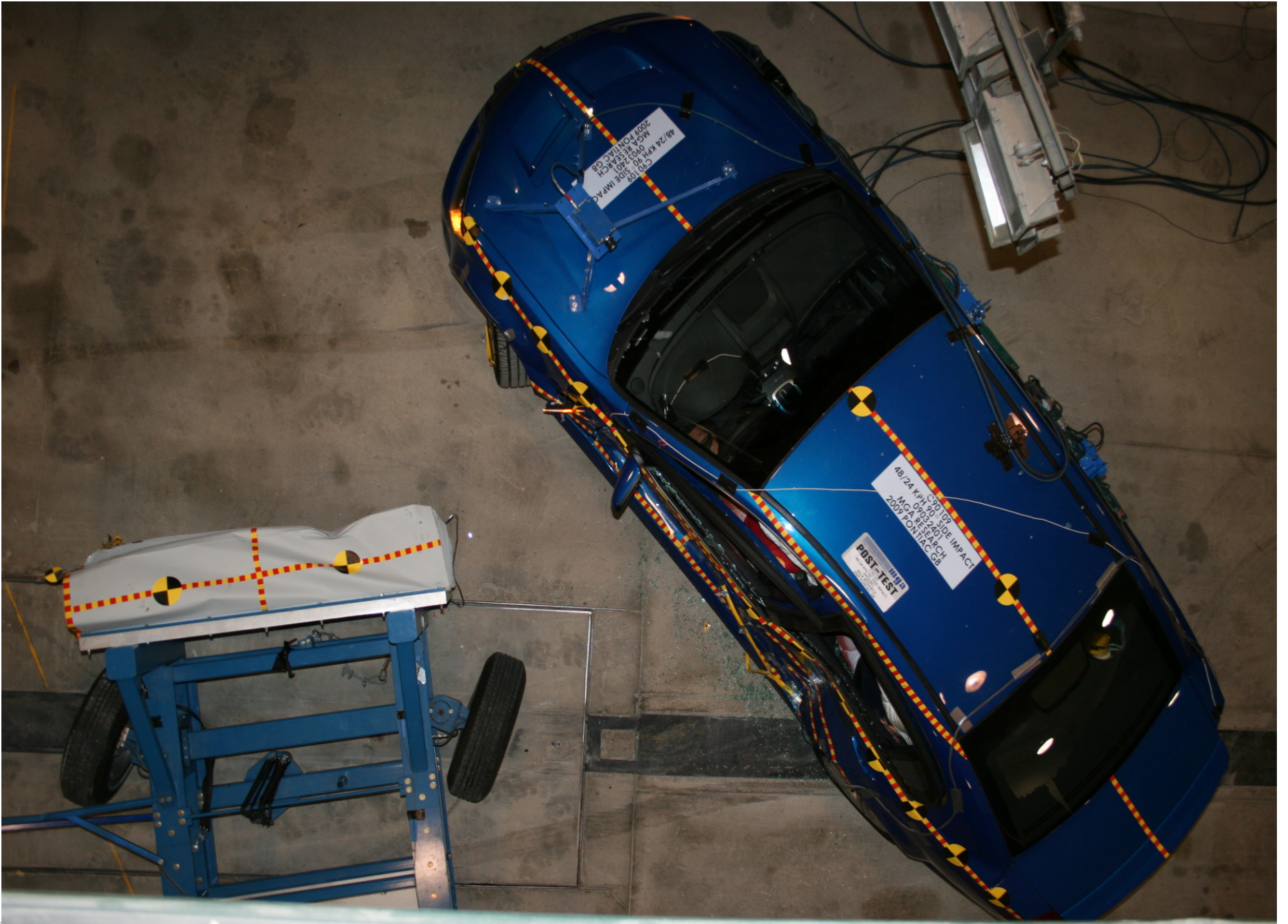
Post-Test MDB and Vehicle Overhead View
